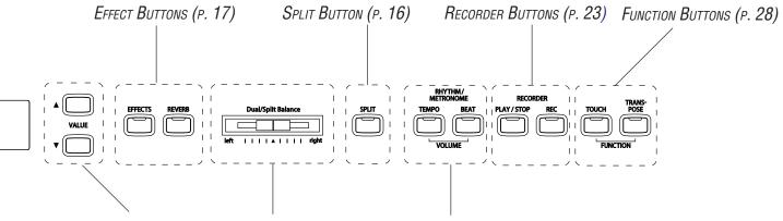
VALUE BUTTONS (P. 15) DUAL/SPLIT BALANCE SLIDER (P.17) METRONOME BUTTONS (P. 20)
